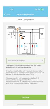
To select the circuit configuration, click the dropdown field. By default, Three Phase Wye Configuration is selected. Currently these are the circuit configuration you can select: Single Phase (2-wire), Single Phase (3-wire) Line-to-Earth, Single Phase (3-wire) Line-to-Line, Three Phase (3-wire) Delta with LineC Earthed, Three Phase (4-wire) Wye Line-to-Neutral and Three Phase (3-Wire) Delta with Mid Tap Connection on A-B.
